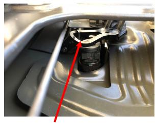
The striker on the solenoid will seat inside this part of the locking mechanism.
