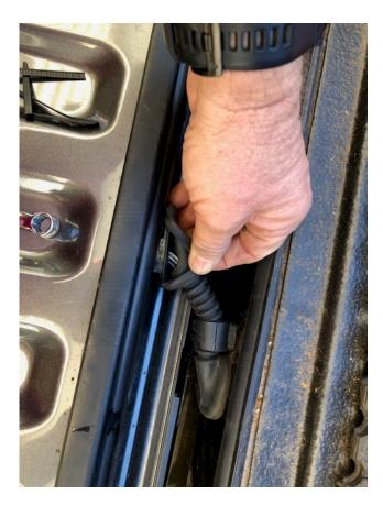
You can pop out the rubber cable tube as shown and feed the new cable through.
