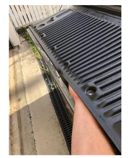
Lower the tailgate and remove the plastic tailgate guard (if fitted) by taking out the T30 Torx screws.
