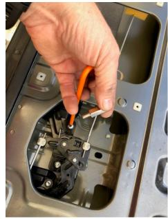
Slide the solenoid mechanism in from the right hand side and make sure the black plastic striker sits within the locking fitting near the key mechanism. You may need to look in on an angle to make sure it is in.
